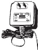
Securitron offers these hard-to-find DC units in two versions: 12 volts@700mA maximum capacity (model PSP-12) and 24 volts@350mA maximum capacity (model PSP-24). They feature an internal thermal fuse and are UL and CSA listed. A 16 ft. output cable is included. They are ideal for powering a wide range of DC devices. Dimensions: 2-1/4" x 2-1/4" x 2-1/2"
