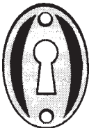
Stock No. PG-75 Finish US-3, 26D Solid brass oval plate with bit key hole. 1-3/4" x 1-1/8" oval escutcheon. Packaged two plates per poly bag.
